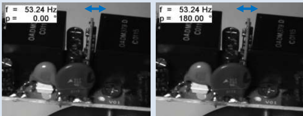
| Movement of electronic components on a PCB board.
